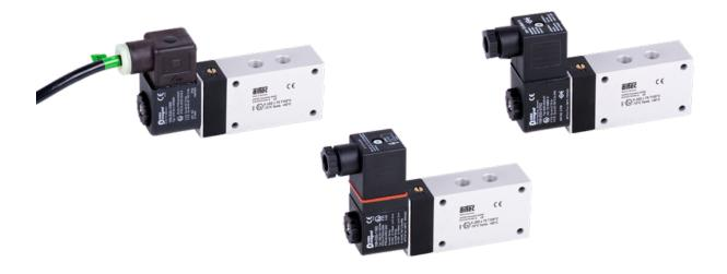
Electrically operated valves conform to equipment category 2 can be used in Zone 1 respectively in Zone 21. For the use in hazardous areas the category group of the used coil has to be taken into account. The specification of the whole equipment corresponds always to the lowest category of the single components.
